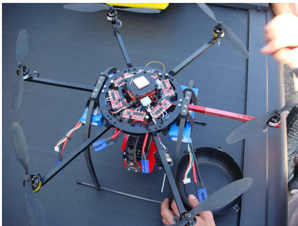
Explorers can have four, six or eight engines depending on the model and desired function. Way points can be programmed so that a specific route is flown with great accuracy and precision. A payload of up to 1kg for the Explorer SH allows it to carry a HD camera or video cam on a gyroscopically stabilised tray for acquisition of the desired high quality vertical or oblique images.
