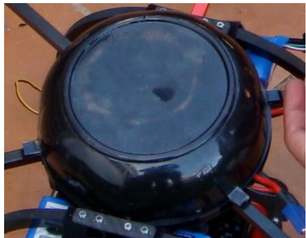
The Explorer's integrated circuitry is contained in a light frame and housed under a custom-made, protective, moulded polycarbonate hemisphere.
